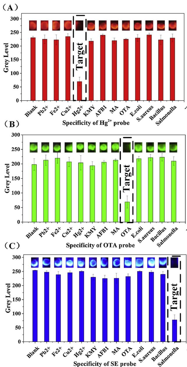
Fig. 4. Specificity evaluation of the developed LFAA. Change in grey level with various types of targets (A) using R-probe, (B) using G-probe and (C) using B-probe. (Concentration was  $10^3$  CFU/mL,  $10 \mu\text{g/mL}$  and  $10^3$  ppb for each bacteria, molecules and ions, respectively.)
