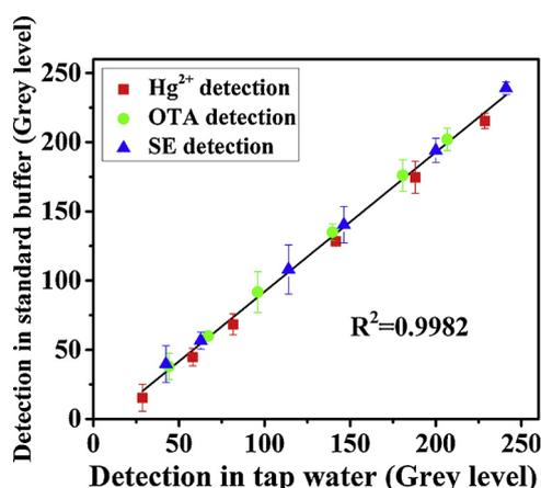
Fig. 6. Correlation between the detection results in the real sample (tap water) and running buffer.
